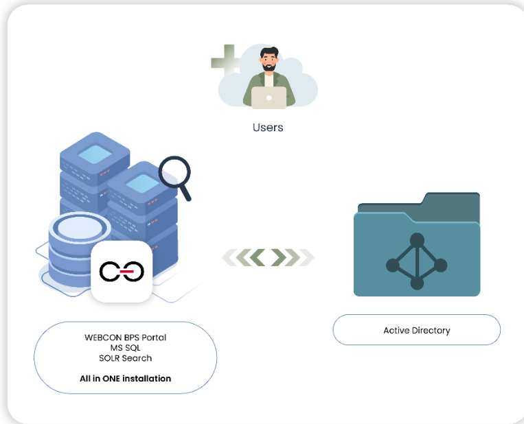
Diagram of „all-in-one“ WEBCON BPS installation
