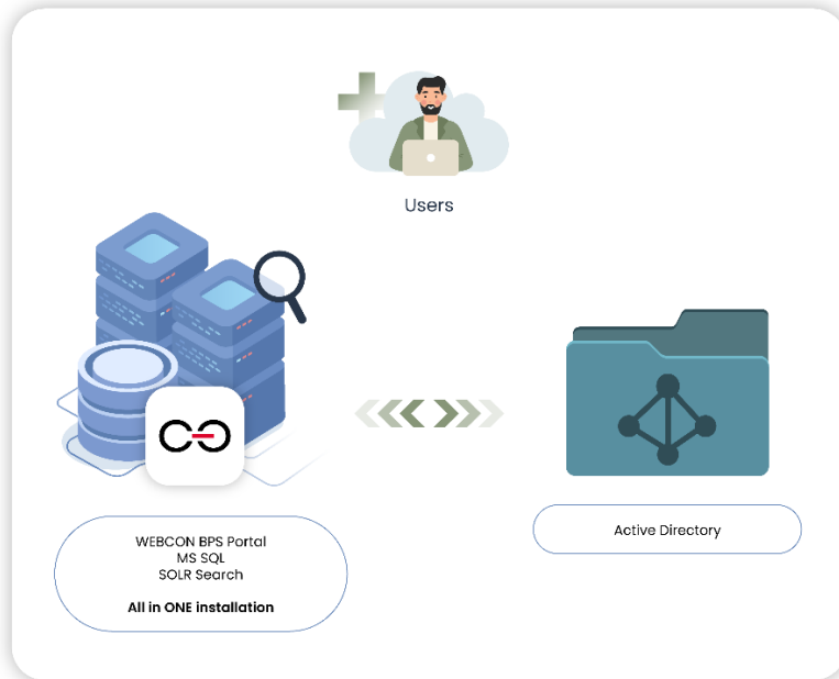
Diagram of „all-in-one” WEBCON BPS installation
