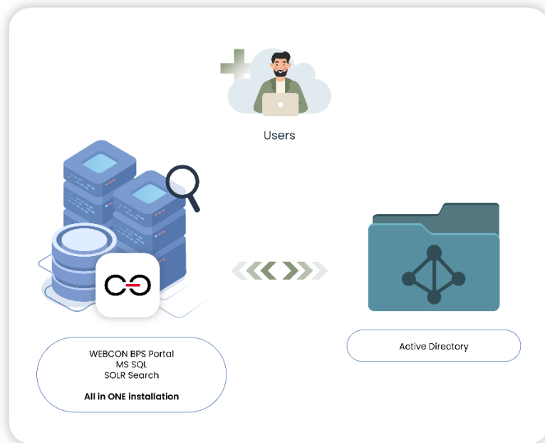
Diagram of „all-in-one“ WEBCON BPS installation
