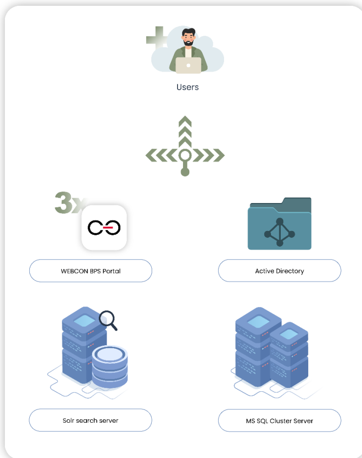
Recommended configuration for WEBCON BPS installation – over 10 000 users
