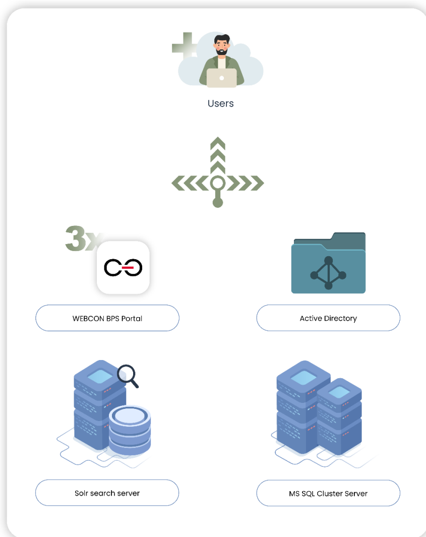
Sample configuration of an environment intended for more than 10 000 users
